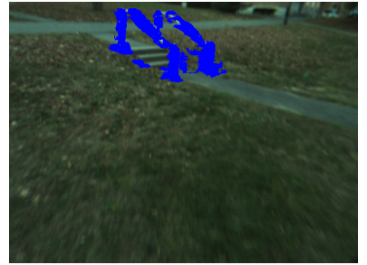
(f) A railing detected as an obstacle.
