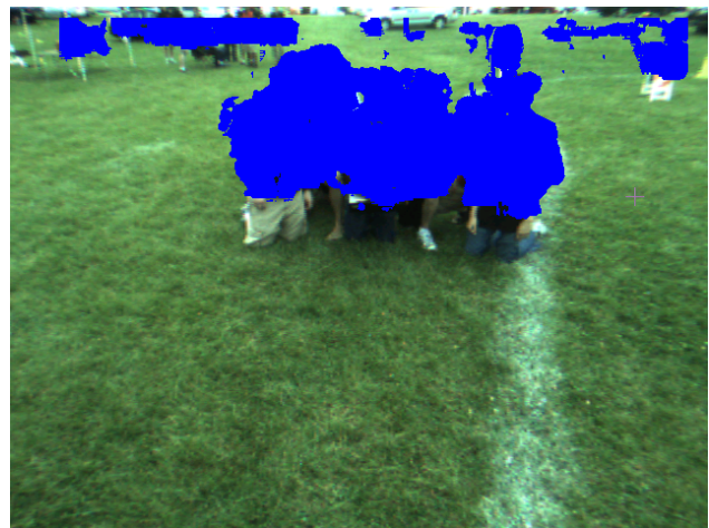
(b) Output of obstacle detection. Pixels detected as obstacles are overwritten in blue.
