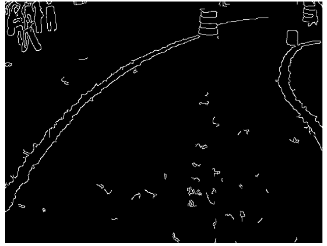
(b) Output of Canny edge detector and horizontal intensity bump filter.
