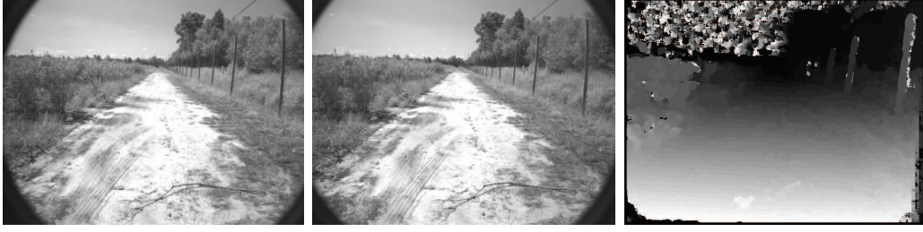
Figure 1.3: The left image, right image, and disparity map for a natural scene
